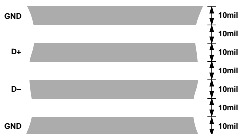
Figure 14. Arrangement of Signal Tracks
