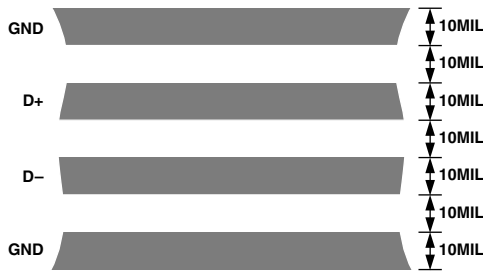
Figure 18. Arrangement of Signal Tracks
