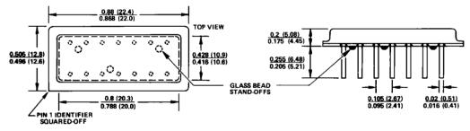
Hermetically sealed 14-Pin Dual-In-Line (Gross leak tested per MIL-STD-883, Method 1014) Pin 7 is electrically connected to the case. Case has metal bottom surface.
