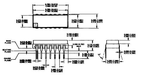
14-Pin Dual-In-Line Ceramic Package
