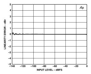
TPC 36. Linearity Error, 48 kHz:48 kHz, 0 dBFS to –140 dBFS Input, 200 Hz Tone
