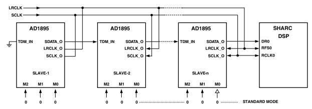
Figure 11. Daisy-Chain Configuration for TDM Mode (All AD1895s Being Clock-Slaves)
