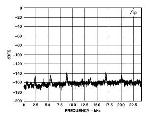
TPC 23. Wideband FFT Plot (16k Points) 96 kHz:48 kHz, 0 dBFS 20 kHz Tone
