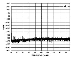
TPC 11. Wideband FFT Plot (16k Points) 44.1 kHz:192 kHz, -60 dBFS 1 kHz Tone
