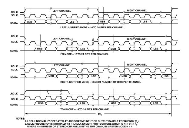
Figure 10. Input/Output Serial Data Formats
