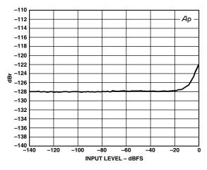
TPC 46. THD + N vs. Input Amplitude, 48 kHz:96 kHz, 1 kHz Tone
