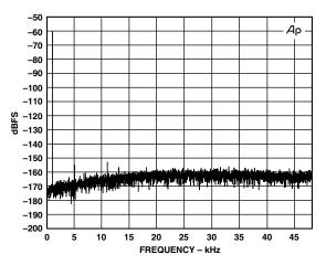
TPC 10. Wideband FFT Plot (16k Points) 48 kHz:96 kHz, -60 dBFS 1 kHz Tone
