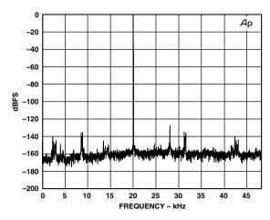
TPC 22. Wideband FFT Plot (16k Points) 48 kHz:96 kHz, 0 dBFS 20 kHz Tone
