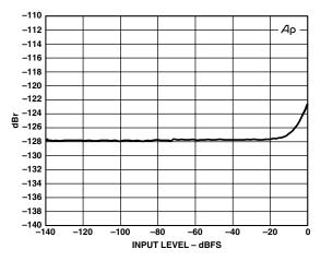
TPC 47. THD + N vs. Input Amplitude, 44.1 kHz:192 kHz, 1 kHz Tone
