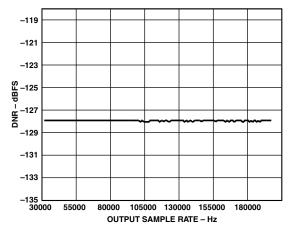
TPC 34. DNR vs. Output Sample Rate,  $f_{S\_IN} = 44.1$  kHz, -60 dBFS 1 kHz Tone
