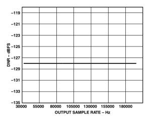
TPC 30. DNR vs. Output Sample Rate,  $f_{S\_IN} = 32 \text{ kHz}$ , -60 dBFS 1 kHz Tone
