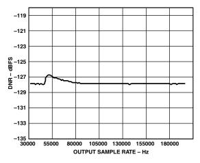
TPC 29. DNR vs. Output Sample Rate,  $f_{S_{\_IN}} = 192 \text{ kHz}$ , -60 dBFS 1 kHz Tone
