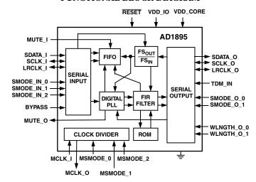
a digital signal processor. The serial output data is dithered down to 20, 18 or 16 bits when 20-, 18- or 16-bit output data is selected. The AD1895 sample rate converts the data from the serial input port to the sample rate of the serial output port. The sample rate at the serial input port can be asynchronous with respect to the output sample rate of the output serial port. The master clock to the AD1895, MCLK, can be asynchronous to both the serial input and output ports.
