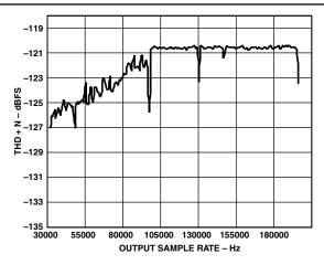
TPC 28. THD + N vs. Output Sample Rate,  $f_{S_{-}|N}$  = 96 kHz, 0 dBFS 1 kHz Tone
