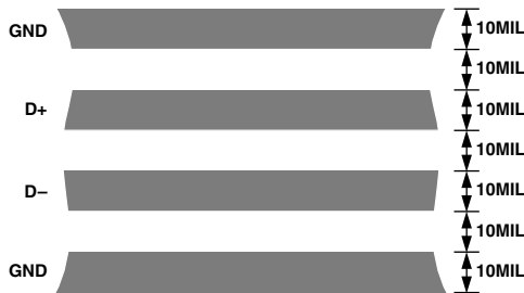
Figure 18. Arrangement of Signal Tracks
