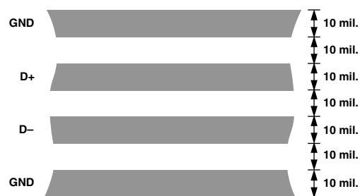
Figure 17. Arrangement of Signal Tracks
