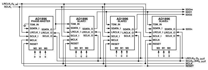
Figure 13. Typical Configuration for Matched Phase Mode Operation
