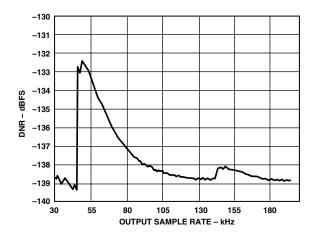
TPC 29. DNR vs. Output Sample Rate,  $f_{S_{-IN}} = 192 \text{ kHz}$ , -60 dBFS 1 kHz Tone
