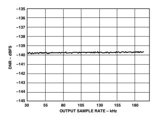
TPC 30. DNR vs. Output Sample Rate,  $f_{S_{_{_{_{}}}N}} = 32 \text{ kHz}$ , -60 dBFS 1 kHz Tone
