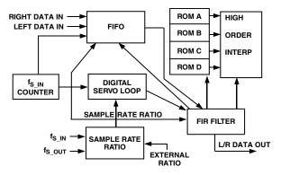
Figure 7. Architecture of the Sample Rate Converter
