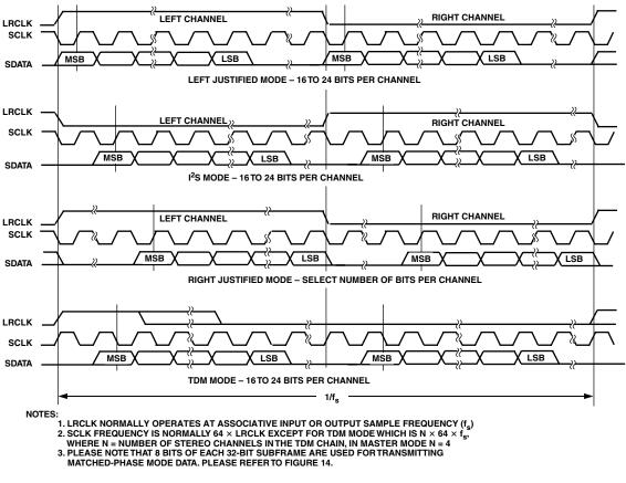
Figure 10. Input/Output Serial Data Formats
