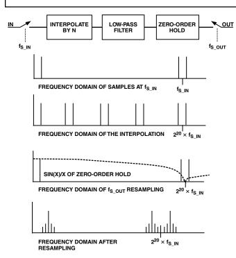
Figure 6. Frequency Domain of the Interpolation and Resampling
