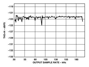
TPC 27. THD + N vs. Output Sample Rate,  $f_{S_{_{_{_{_{}}}N}}} = 32 \text{ kHz}$ , 0 dBFS 1 kHz Tone
