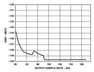
TPC 31. DNR vs. Output Sample Rate,  $f_{S_{-}IN} = 96 \text{ kHz}$ , -60 dBFS 1 kHz Tone
