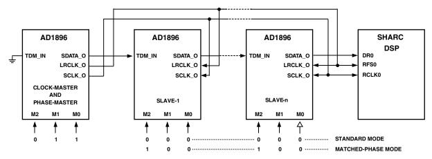
Figure 12. Daisy-Chain Configuration for TDM Mode (First AD1896 Being Clock-Master)
