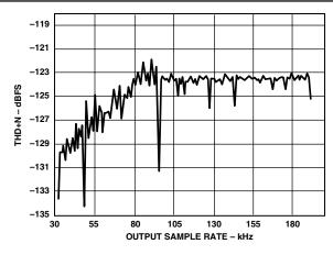
TPC 28. THD + N vs. Output Sample Rate,  $f_{S_{_{_{_{}}}N}} = 96 \text{ kHz}$ , 0 dBFS 1 kHz Tone
