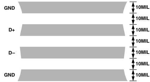
Figure 4. Arrangement of Signal Tracks
