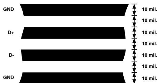
Figure 10. Arrangement of Signal Tracks
