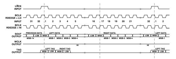
Figure 15. Serial Data Output Timing: Slave Mode, Left-Justified with No MSB Delay, 32-Bit Frame Mode,  $S\overline{M} = HI$ ,  $R\overline{L}JUST = LO$ ,  $\overline{MSBDLY} = HI$
