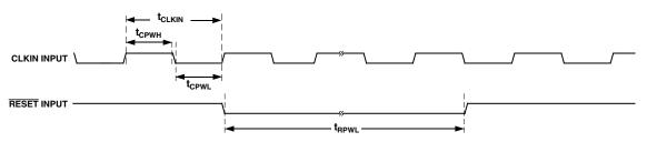
Figure 19. CLKIN and RESET Timing
