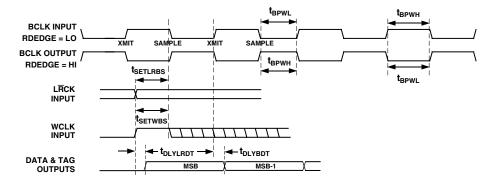
Figure 18. Slave Mode Clock Timing
