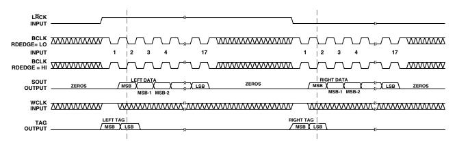
Figure 8. Serial Data Output Timing: Slave Mode, Data Position Controlled by WCLK Input,  $S\overline{M} = HI$ ,  $R\overline{L}JUST = HI$ ,  $\overline{MSBDLY} = LO$
