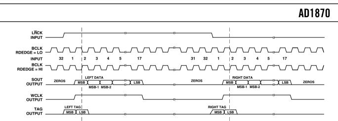
Figure 10. Serial Data Output Timing: Slave Mode,  $l^2S$ -Justified,  $S\overline{M} = HI$ ,  $R\overline{L}JUST = LO$ ,  $\overline{MSBDLY} = LO$
