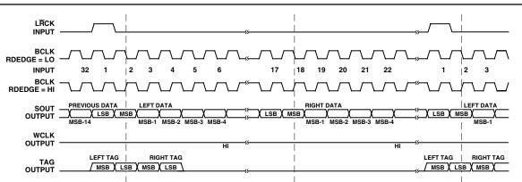
Figure 16. Serial Data Output Timing: Slave Mode,  $I^2S$ -Justified, 32-Bit Frame Mode,  $S\overline{M} = HI$ ,  $R\overline{L}JUST = LO$ ,  $\overline{MSBDLY} = LO$
