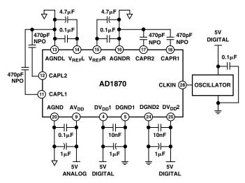
Figure 3. Recommended Bypassing and Oscillator Circuits
