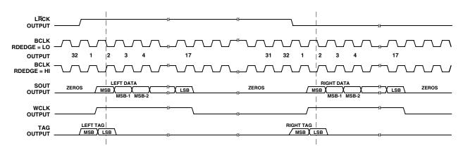
Figure 14. Serial Data Output Timing: Master Mode,  $l^2S$ -Justified,  $S\overline{M} = LO$ ,  $R\overline{L}JUST = LO$ ,  $\overline{MSBDLY} = LO$
