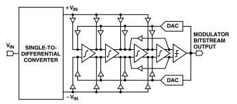
Figure 1. Modulator Noise-Shaper (One Channel)
