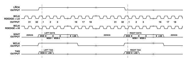
Figure 13. Serial Data Output Timing: Master Mode, Left-Justified with No MSB Delay,  $S\overline{M} = LO$ ,  $R\overline{L}JUST = LO$ ,  $\overline{MSBDLY} = HI$
