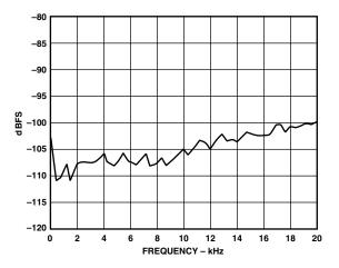
TPC 6. Channel Separation vs. Frequency at -0.5 dBFS
