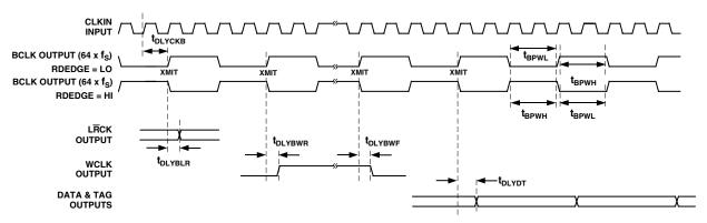
Figure 17. Master Mode Clock Timing
