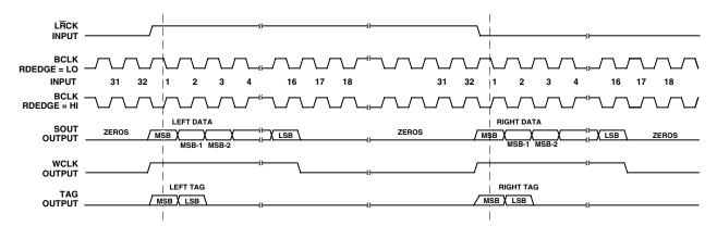
Figure 9. Serial Data Output Timing: Slave Mode, Left-Justified with No MSB Delay,  $S\overline{M} = HI$ , RLJUST = LO,  $\overline{MSBDLY} = HI$
