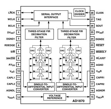
one-bit comparator's quantization noise out of the audio passband. The high order of the modulator randomizes the modulator output, reducing idle tones in the AD1870 to very low levels. Because its modulator is single-bit, the AD1870 is inherently monotonic and has no mechanism for producing differential linearity errors.
