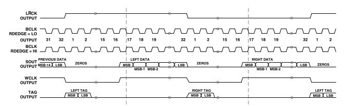
Figure 11. Serial Data Output Timing: Master Mode, Right-Justified with No MSB Delay,  $S\overline{M} = LO$ ,  $R\overline{L}JUST = HI$ ,  $\overline{MSBDLY} = HI$
