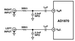
*Figure 2. Recommended Input Structure for Externally DC-Coupled Inputs*
