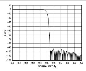
TPC 7. Digital Filter Signal Transfer Function to f<sub>S</sub>
