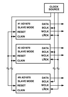
Figure 6. Synchronizing Multiple AD1870s
