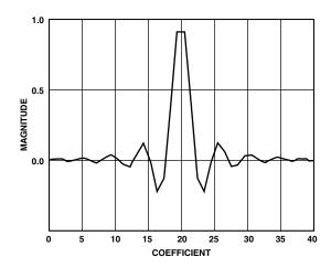
Figure 37. Typical Impulse Response for WBCDMA
