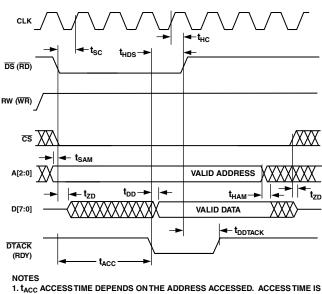
t<sub>ACC</sub> ACCESS TIME DEPENDS ON THE ADDRESS ACCESSED. ACCESS TIME IS MEASURED FROM FE OF DS TO THE FE OF DTACK.
