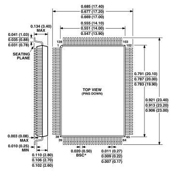
\* THE ACTUAL POSITION OF EACH LEAD IS WITHIN 0.00315 (0.08) FROM ITS IDEAL POSITION WHEN MEASURED IN THE LATERAL DIRECTION. CENTER FIGURES ARE TYPICAL UNLESS OTHERWISE NOTED
