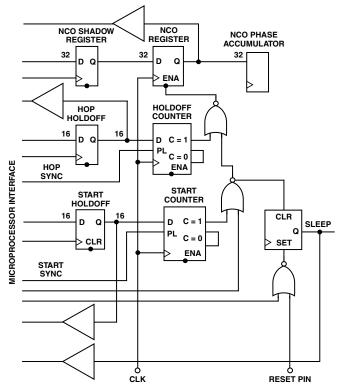
Figure 34. NCO Shadow Register and Hold-Off Counter
