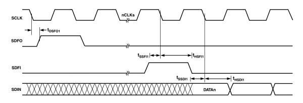
Figure 11. Serial Port Timing, Slave Mode (SCS = 1), Channel is External-Framing
