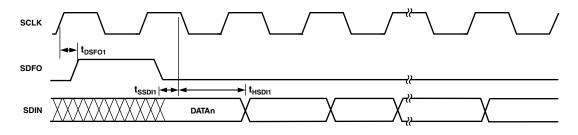
Figure 9. Serial Port Timing, Slave Mode (SCS = 1), Channel is Self-Framing
