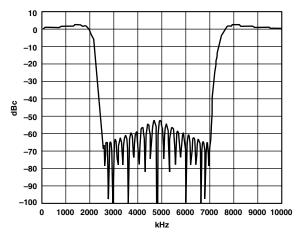
Figure 38. RAM Coefficient Filter, Frequency Response for WBCDMA
