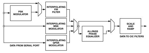
Figure 18. RCF Block Diagram
