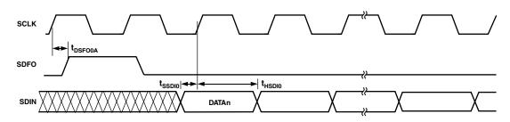
Figure 8. Serial Port Timing, Master Mode (SCS = 0), Channel is Self-Framing
