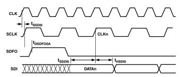
Figure 16. Serial Port Switching Characteristics
