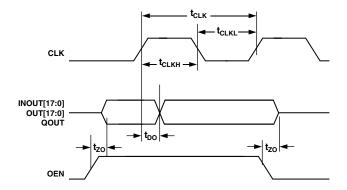
Figure 1. Parallel Output Switching Characteristics
