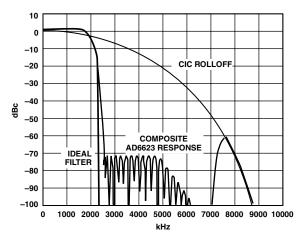
Figure 39. RCF and CIL, Frequency Response for WBCDMA
