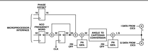
Figure 31. Numerically Controlled Oscillator and QAM Mixer
