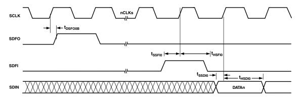
Figure 10. Serial Port Timing, Master Mode (SCS = 0), Channel is External-Framing
