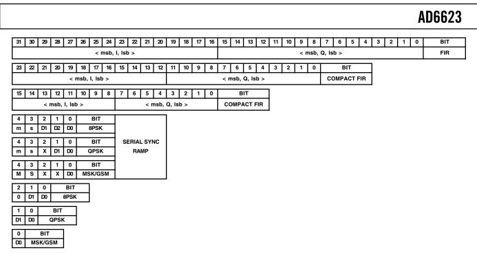
Figure 17. Data Formats Supported by the AD6623 when SCLK Master (SCS = 0), and SFDO Set for Frame Request (SFE = 0)
