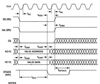
$t_{ACC}$  ACCESS TIME DEPENDS ON THE ADDRESS ACCESSED. ACCESS TIME IS MEASURED FROM FE OF  $\overline{DS}$  TO THE FE OF  $\overline{DTACK}.$
