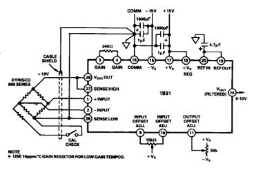
Figure 16. Pressure Transducer Application
