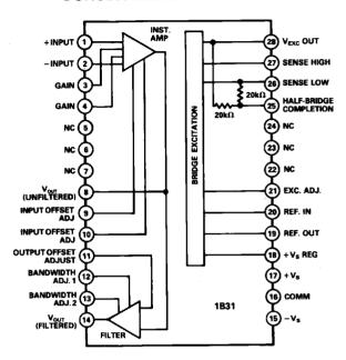
pair of thin-film  $20k\Omega$  resistors is connected across the excitation outputs. This assures temperature tracking of ±5ppm/°C max and reduces part count.
