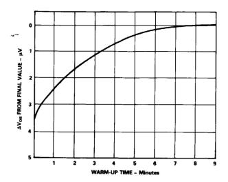
Figure 12. Offset Voltage, RTI, Turn-On Drift
