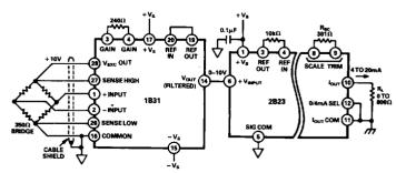
Figure 20. Isolated 4-20mA Transmitter
