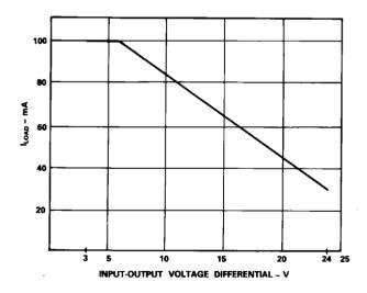
Figure 13. Excitation Source Input – Output Voltage Differential vs. Load Current; Ambient Temperature ≤25°C.
