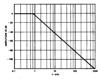
Figure 9. Filter Amplitude Response vs. Frequency
