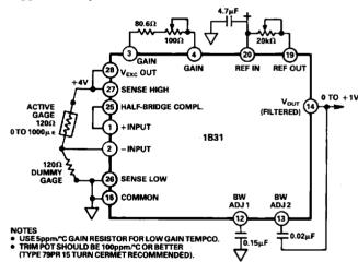
Figure 15. Strain Gage Application Using Internal Half-Bridge
