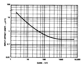
Figure 8. Total Input Offset Drift vs. Gain
