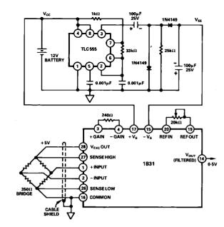
Figure 18. Negative Supply Generation for 1B31
