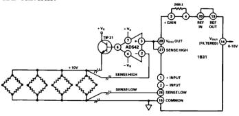
Figure 17. Multiple Load-Cell Application
