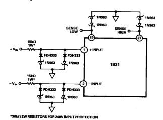
Figure 7. 115V Input Protection for 1B31
