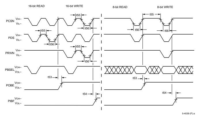
Figure 25. PHIF Motorola Mode Signaling (Pulse Period and Flags) Timing Diagram
