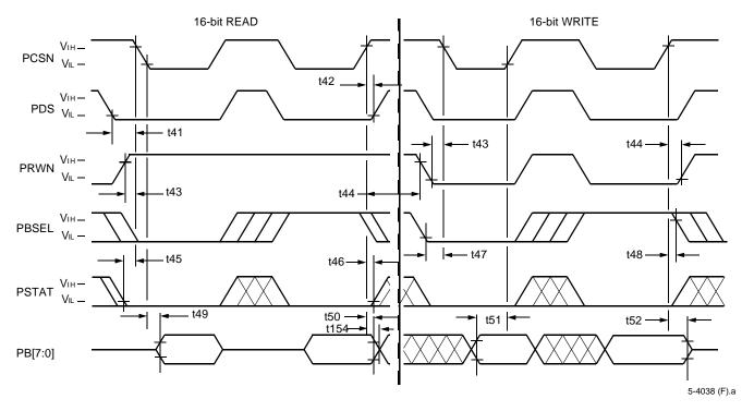
Figure 72. PHIF Motorola Mode Signaling (Read and Write) Timing Diagram
