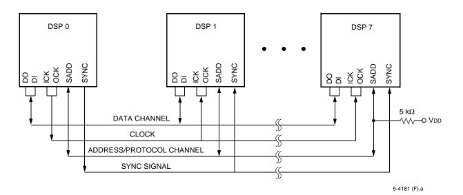
Figure 5. Multiprocessor Communication and Connections
