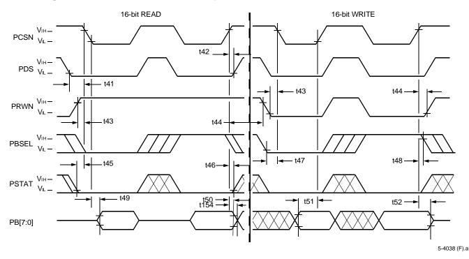
Figure 48. PHIF Motorola Mode Signaling (Read and Write) Timing Diagram
