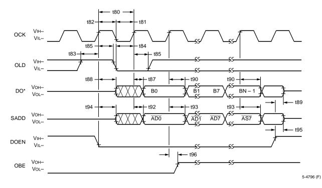
\* See sioc register, MSB field to determine if B0 is the MSB or LSB. See sioc register, ILEN field to determine if the DO word length is 8 bits or 16 bits.
