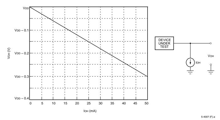
Figure 9. Plot of VOH vs. IOH Under Typical Operating Conditions
