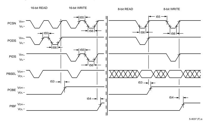
Figure 71. PHIF Intel Mode Signaling (Pulse Period and Flags) Timing Diagram
