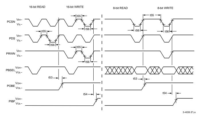
Figure 73. PHIF Motorola Mode Signaling (Pulse Period and Flags) Timing Diagram
