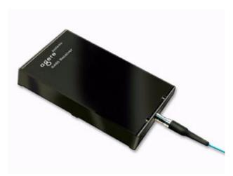
Manufactured in a low-profile, 24-pin package, the R480-Type receiver features either an avalanche or PIN photodetector, a transimpedance amplifier, and a limiting amplifier IC.
