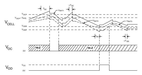
• Overcurrent Protection (V<sub>CELL</sub>=3.5V)
