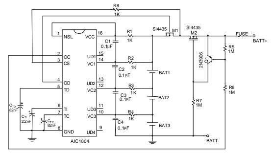
Fig. 1 Protection Circuit for Three-Cell Lithium-Ion Battery Pack
