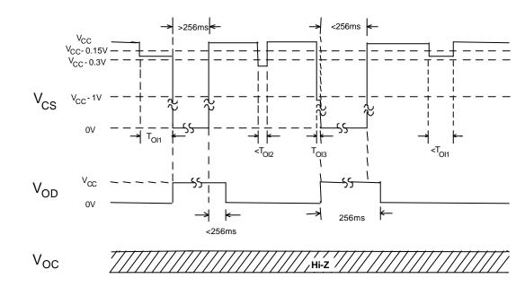
• Overcurrent Protection (V<sub>CELL</sub>=3.5V)
