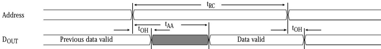
Read waveform 2 (chip selects,  $\overline{OE}$ ,  $\overline{UB}$ ,  $\overline{LB}$  controlled)
