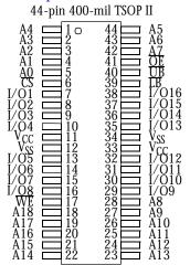
Note: A "MODE" pad is to be placed between pins 33 and 34 and 11 and 12, shorted. The bonding of this pad to  $V_{CC}$  or  $V_{SS}$  configures the device. There should only be 44+2+2 pads on the chip. Two extra  $V_{CC}$  to separate out Array from Peripheral and Two-Mode Pads.
