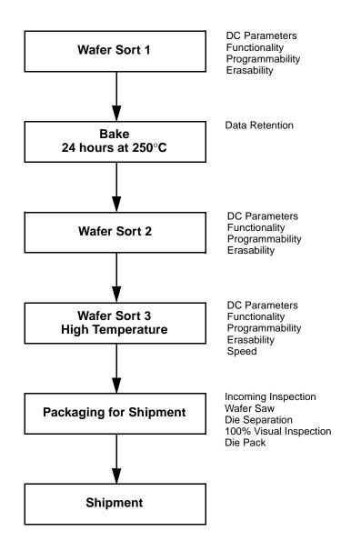
Figure 1. AMD KGD Product Test Flow
