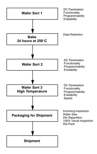
Figure 1. AMD KGD Product Test Flow
