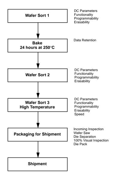
Figure 1. AMD KGD Product Test Flow
