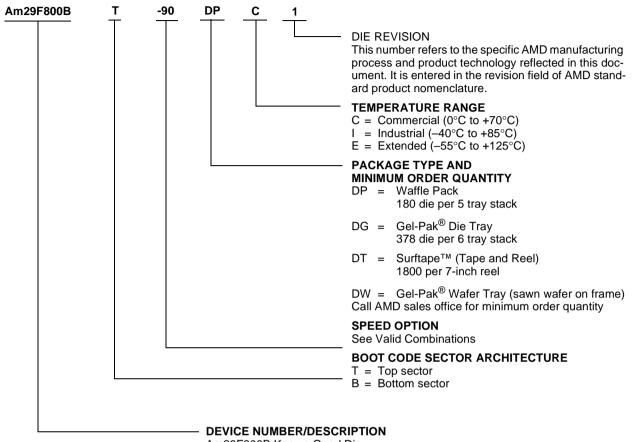
Am29F800B Known Good Die 8 Megabit (1 M x 8-Bit/512 K x 16-Bit) CMOS Flash Memory—Die Revision 1 5.0 Volt-only Program and Erase
