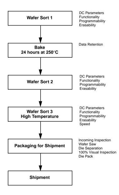
Figure 1. AMD KGD Product Test Flow
