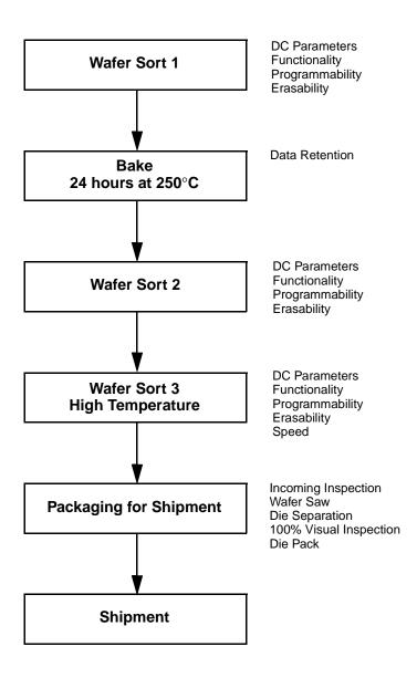
Figure 1. AMD KGD Product Test Flow
