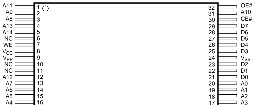
32-Pin — Standard Pinout
