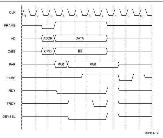
Figure 11. Slave Cycle Data Parity Error Response
