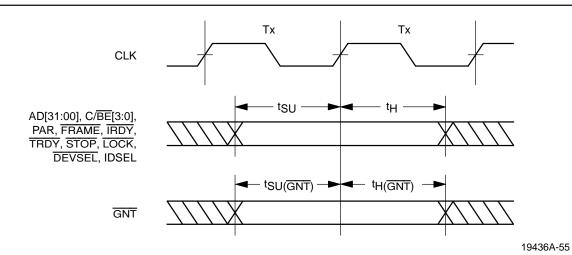
**Input Setup and Hold Timing**
