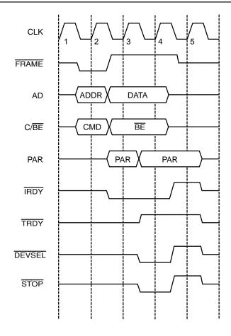
Figure 6. Disconnect Of Slave Cycle When Busy
