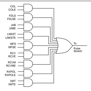
Figure 41. LED Control Logic
