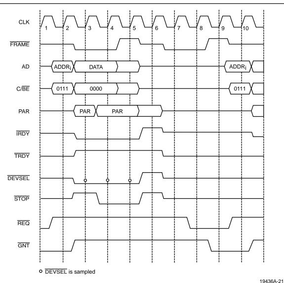
Figure 18. Disconnect Without Data Transfer
