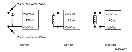
The most critical pins in the layout of a PCnet-PCI II design are the 4 analog power and 2 analog ground pins, AVDD[1–4] and AVSS[1–2], respectively. All of these pins are located in one corner of the device, the "analog corner." Specific functions and layout requirements of the analog power and ground pins are given below.
