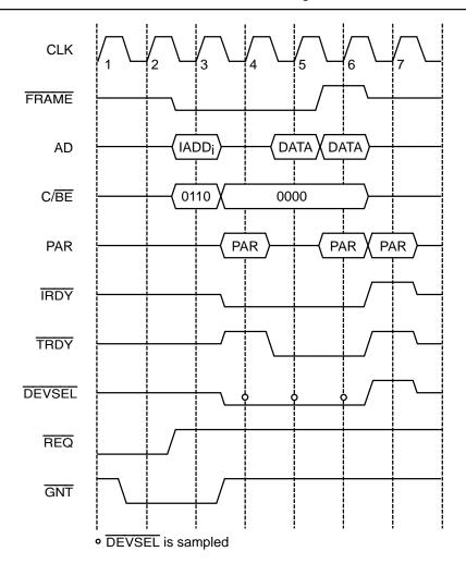
Figure 25. Initialization Block Read In Burst Mode
