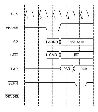
Figure 10. Address Parity Error Response
