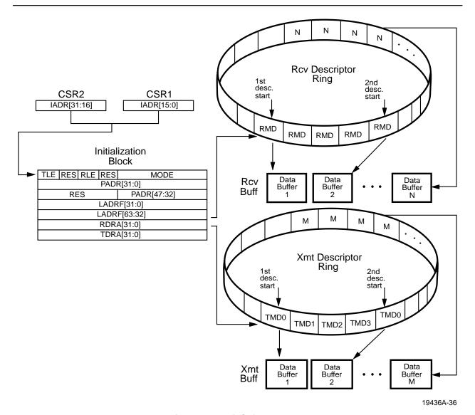
Figure 33. 32-bit Software Model
