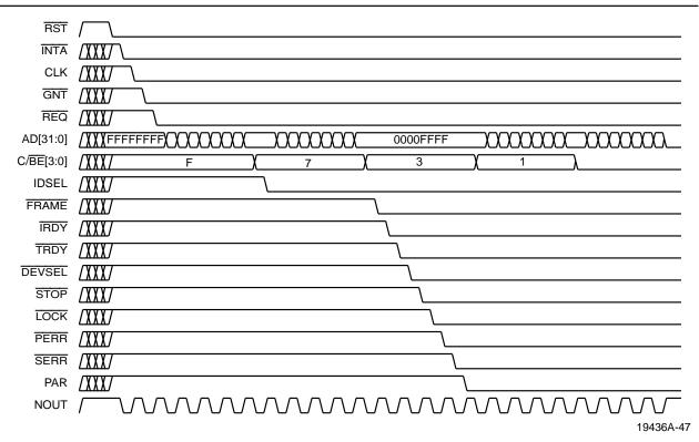
Figure 1. NAND Tree Waveform
