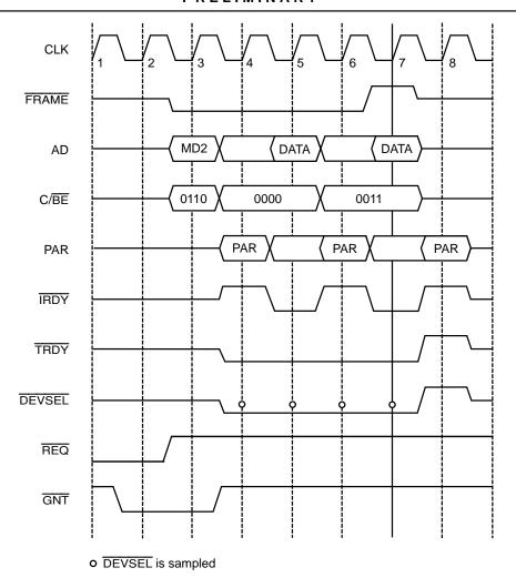
Figure 29. Descriptor Ring Write In Burst Mode
