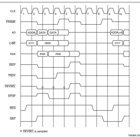
Figure 17. Disconnect With Data Transfer
