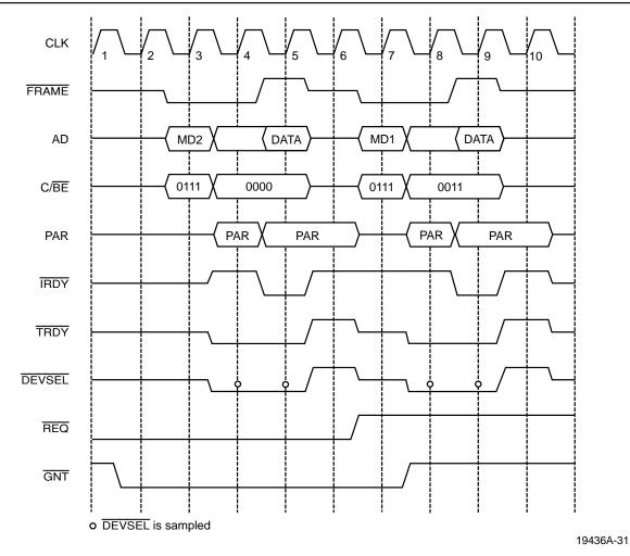
Figure 28. Descriptor Ring Write In Non-Burst Mode
