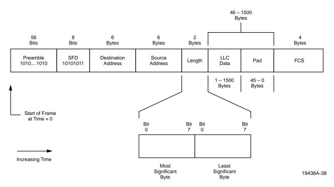
Figure 35. 802.3 Frame And Length Field Transmission Order
