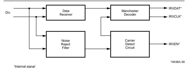
Figure 36. Receiver Block Diagram
