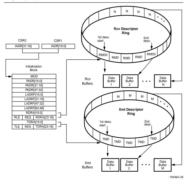
Figure 32. 16-Bit Software Model
