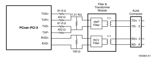
Figure 38. 10BASE-T Interface Connection
