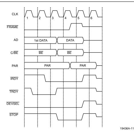
Figure 8. Disconnect Of Slave Burst Transfer—Host Inserts Wait States
