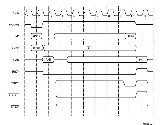
Figure 3. Slave Read Using I/O Command
