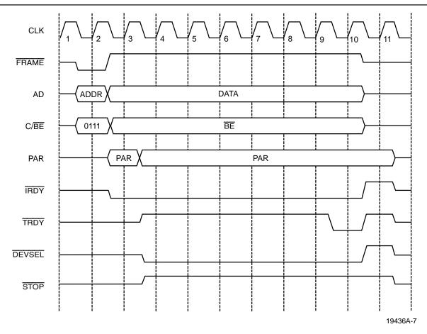
Figure 4. Slave Write Using Memory Command
