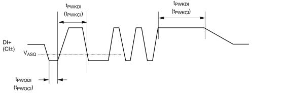
Figure 22. AUI Receive Diagram
