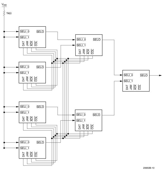
Figure 5. Internal Arbitration—eIMR Devices in Cascade
