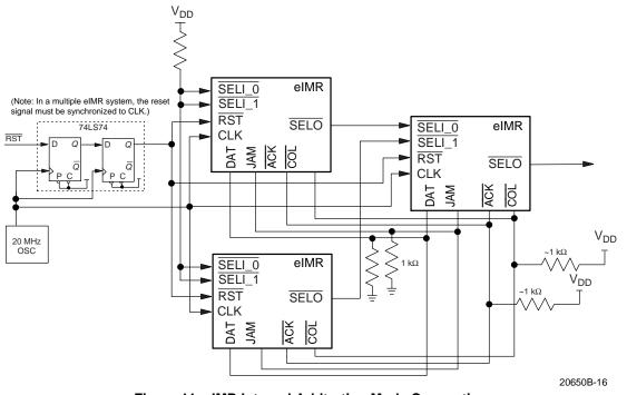
Figure 11. eIMR Internal Arbitration Mode Connection
