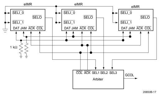
Figure 12. IMR+ Mode External Arbitration
