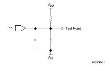
Figure 26. Switching Test Circuit
