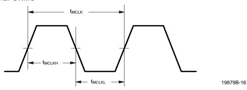
Figure 12. Master Clock (MCLK) Timing
