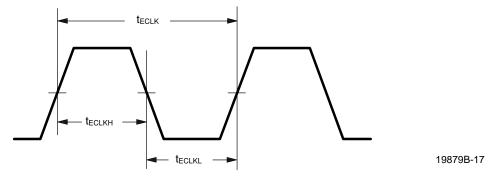
Figure 13. Expansion Bus Asynchronous Clock (ECLK) Timing
