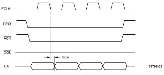
Figure 19. Expansion Port Output Timing - Asynchronous Mode
