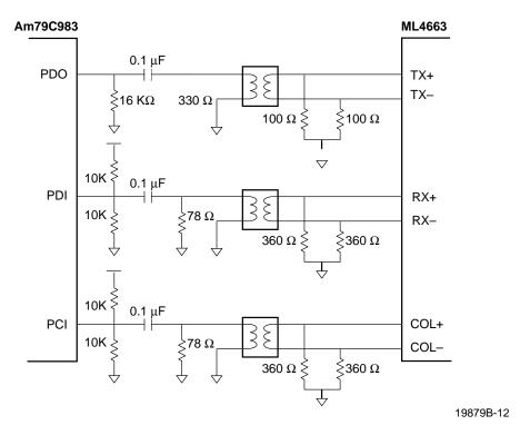
Figure 8. PAUI Interface to non-QuIET Device Transceiver
