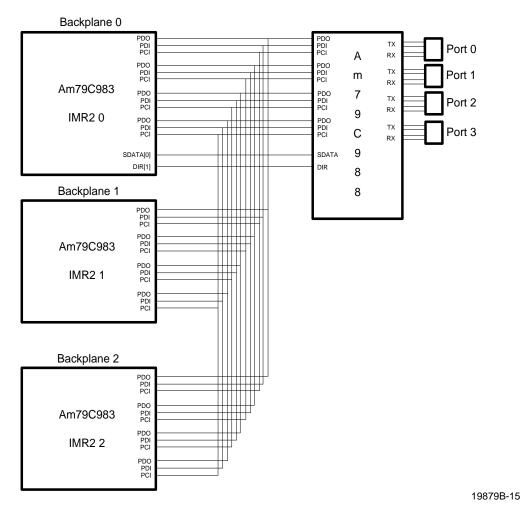
Figure 11. Port Switching Configuration
