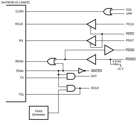
Figure 10. PR Port Connection to an Am79C90 C-Lance
