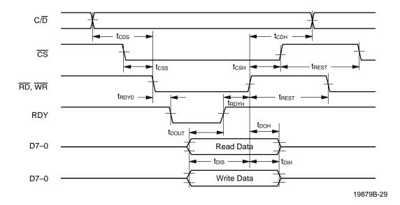
Figure 25. Microprocessor Bus Interface Timing
