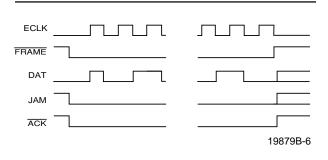
Figure 2. Asynchronous Mode Data Transfer
