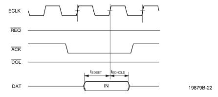
Figure 18. Expansion Port Input Timing - Asynchronous Mode
