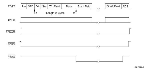
Figure 4. Packet Port Signals
