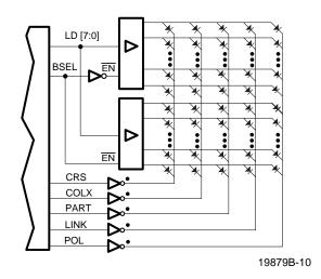
Figure 6. Visual Monitoring Application - Simplified Schematic
