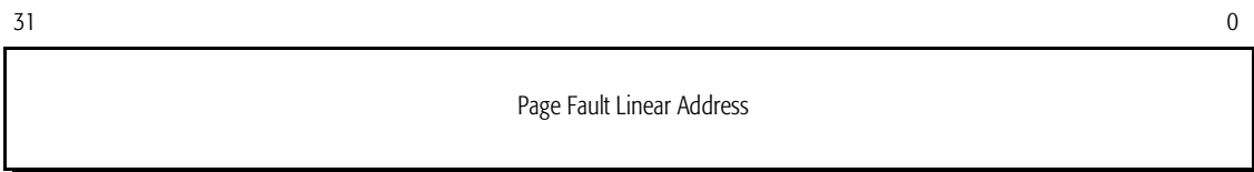
Figure 21. Control Register 2 (CR2)
