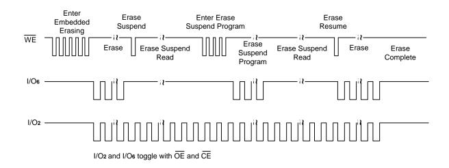
Note: Both I/Os and I/O2 toggle with OE or CE. See the text on I/Os and I/O2 in the section "Write Operation Statue" for more information.
