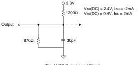
(Fig. 1) DC Output Load Circuit
