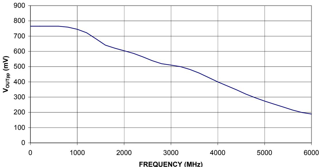
\*Measured using a 750mV differential input source at 50% duty cycle.
