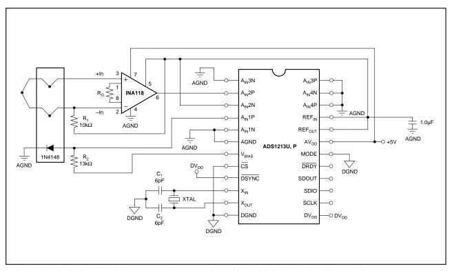
FIGURE 43. Single Supply, High Accuracy Thermocouple Interface with Cold Junction Compensation.
