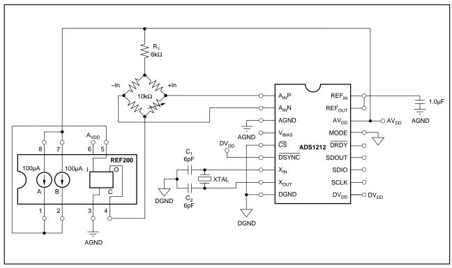
FIGURE 45. Low Cost Bridge Transducer Interface with Current Excitation.
