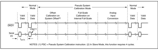
FIGURE 8. Pseudo System Calibration Timing.
