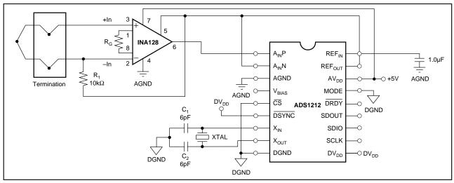
FIGURE 41. Single Supply, High Accuracy Thermocouple.
