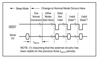
FIGURE 10. Sleep Mode to Normal Mode Timing.
