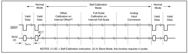
FIGURE 5. Self-Calibration Timing.
