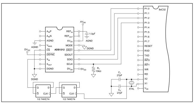
FIGURE 30. Four-Wire Interface with a 8xC32 Microprocessor.
