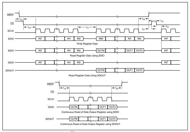
FIGURE 19. Serial Interface Timing (Using  $\overline{\text{CS}}$ ), Slave Mode.
