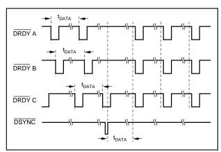
FIGURE 36. Affect of Synchronization on Output Data Timing.
