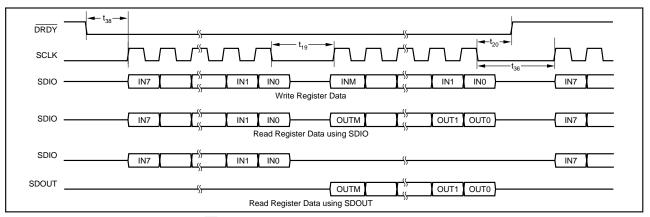
FIGURE 17. Serial Interface Timing ( $\overline{\text{CS}}$  LOW), Slave Mode.
