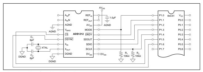
FIGURE 31. Full Interface with a 8xC51 Microprocessor.
