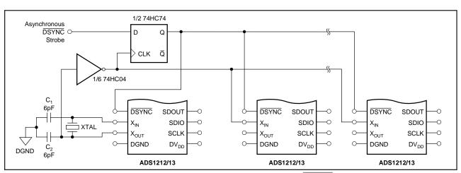
FIGURE 23. Exactly Synchronizing Multiple ADS1212/13s to an Asynchronous DSYNC Signal.
