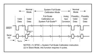
FIGURE 7. System Full-Scale Calibration Timing.
