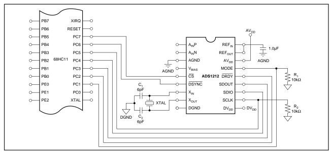
FIGURE 32. Full Interface with a 68HC11 Microprocessor.
