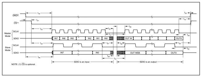
FIGURE 20. SDIO Input to Output Transition Timing.
