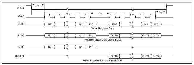
FIGURE 16. Serial Interface Timing ( $\overline{\text{CS}}$  LOW), Master Mode.
