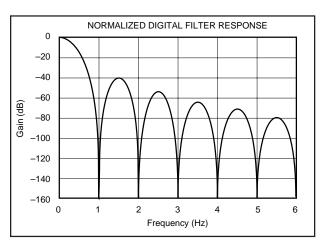
FIGURE 1. Normalized Digital Filter Response.
