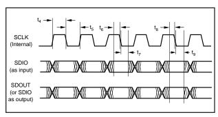
FIGURE 14. Serial Input/Output Timing, Master Mode.
