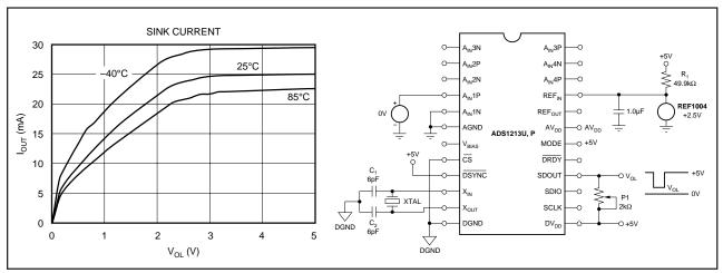
FIGURE 35. Sink Current vs V<sub>OL</sub> for SDOUT Under Worst-Case Conditions.
