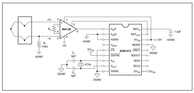
FIGURE 42. Dual Supply, High Accuracy Thermocouple.
