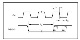
FIGURE 22.  $\overline{DSYNC}$  to  $X_{IN}$  Timing for Synchronizing Mutliple ADS1212/13s.
