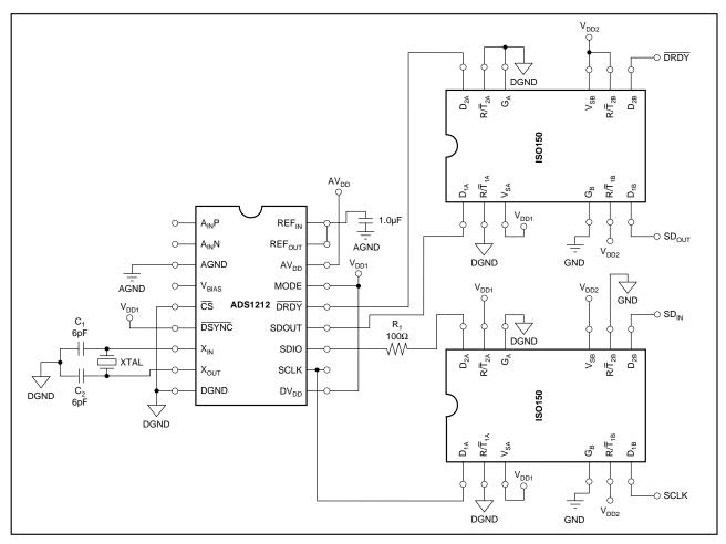
FIGURE 33. Isolated Four-Wire Interface.
