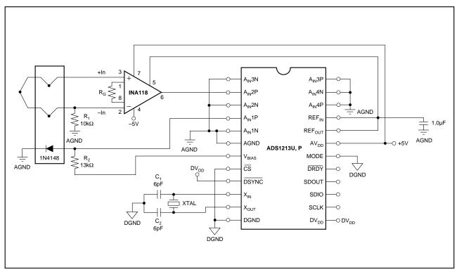
FIGURE 44. Dual Supply, High Accuracy Thermocouple Interface with Cold Junction Compensation.
