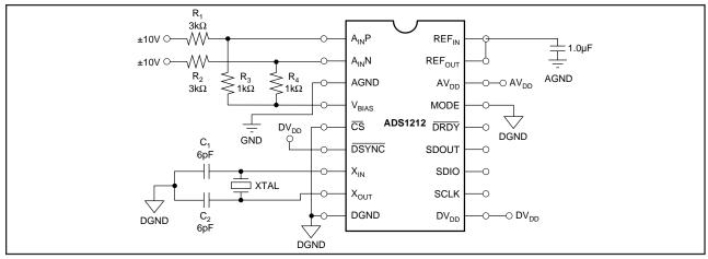
FIGURE 12. ±10V Input Configuration Using V<sub>BIAS</sub>.
