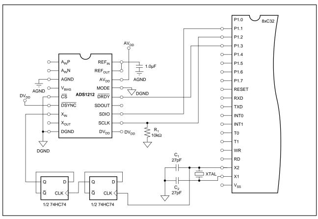
FIGURE 28. Three-Wire Interface with a 8xC32 Microprocessor.
