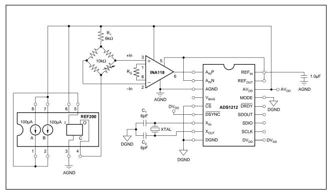
FIGURE 38. Bridge Transducer Interface with Current Excitation.
