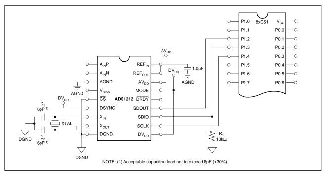
FIGURE 29. Three-Wire Interface with a 8xC51 Microprocessor.
