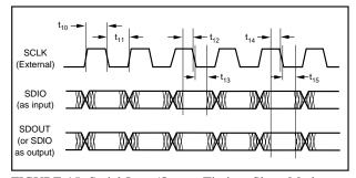
FIGURE 15. Serial Input/Output Timing, Slave Mode.
