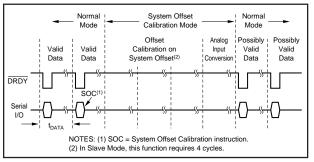
FIGURE 6. System Offset Calibration Timing.
