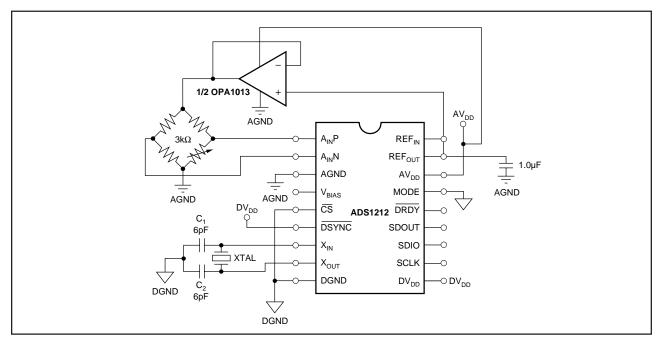
FIGURE 37. Bridge Transducer Interface with Voltage Excitation.
