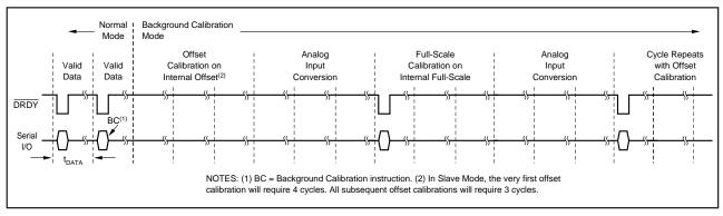
FIGURE 9. Background Calibration Timing.
