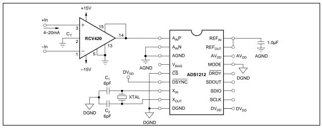
FIGURE 40. Complete 4-20mA Receiver.
