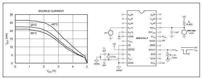
FIGURE 34. Source Current vs V<sub>OH</sub> for SDOUT Under Worst-Case Conditions.
