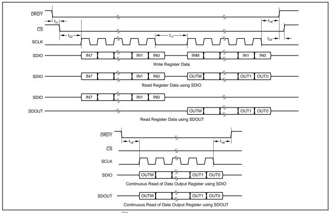
FIGURE 18. Serial Interface Timing (Using  $\overline{CS}$ ), Master Mode.
