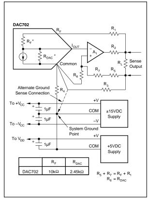
FIGURE 8. Differential Sensing Output Op Amp Configuration.
