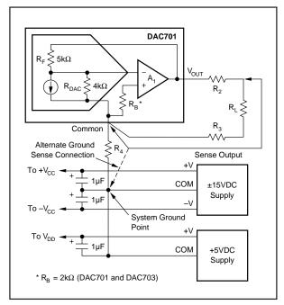
FIGURE 6. Output Circuit for Voltage Models.
