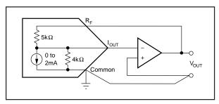
FIGURE 9. External Op Amp Using Internal Feedback
