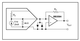
FIGURE 11. External Op Amp Using External Feedback Resistors.
