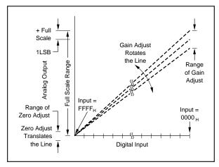
FIGURE 4. Relationship of Zero and Gain Adjustments for Unipolar D/A Converters, DAC701.
