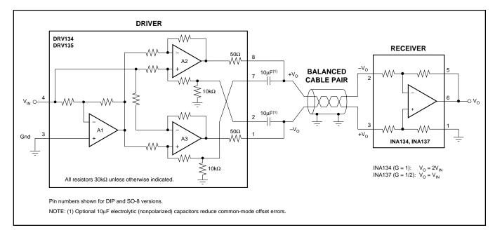
FIGURE 2. Complete Audio Driver/Receiver Circuit.
