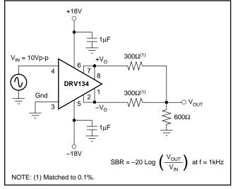
FIGURE 5. Signal Balance Ratio Test Circuit.
