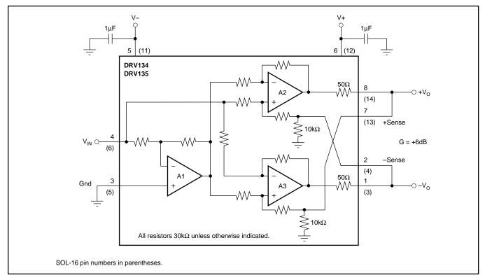
FIGURE 1. Basic Connections.
