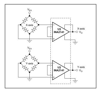
FIGURE 4. Two-Axis Bridge Amplifier.
