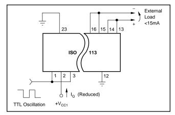
FIGURE 5. Reduced Power Dissipation.
