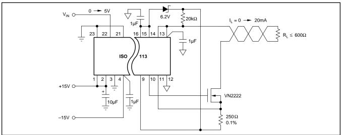
FIGURE 6. Isolated Current Loop Driver.
