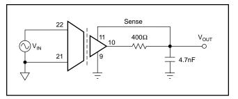
FIGURE 4. Ripple Reduction.
