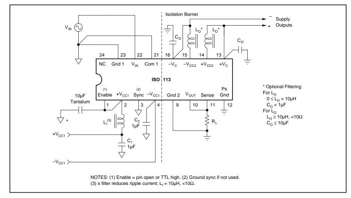
FIGURE 1. Signal and Power Connections.
