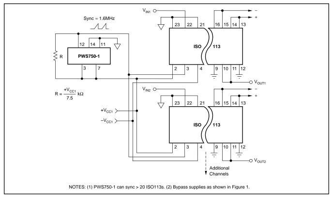
FIGURE 7. Synchronized-Multichannel Isolation.
