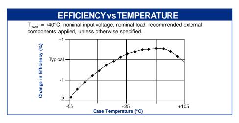
$\begin{tabular}{ll} SPECIFICATIONS, ALL MODELS \\ Specifications are at $T_{CASE}$ = +40 °C nominal input voltage unless otherwise specified. \\ \end{tabular}$
