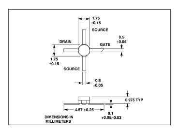
base station receiver in PCS, Japanese PHS, AMPS, GSM and other communications systems. The CFB0301 is in an industry-standard 70 mil package. It is surface mountable and available in tape and reel.
