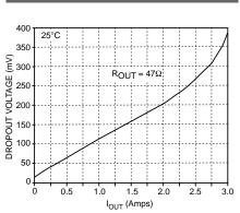
Dropout Voltage vs. I<sub>OUT</sub>
