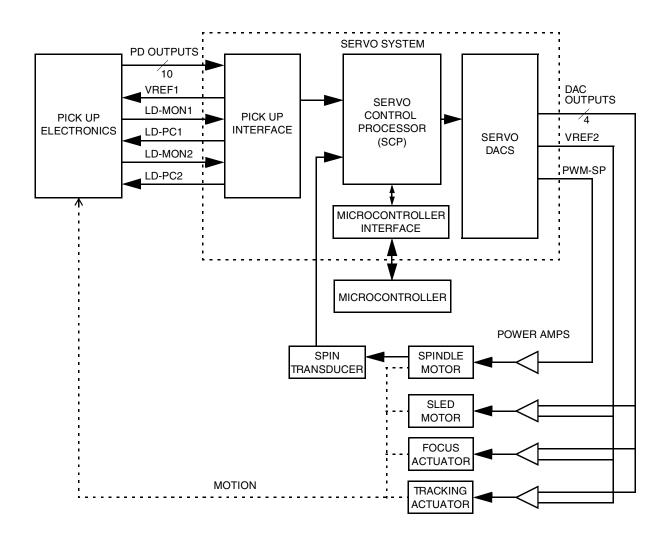
Figure 2. Servo System Diagram
