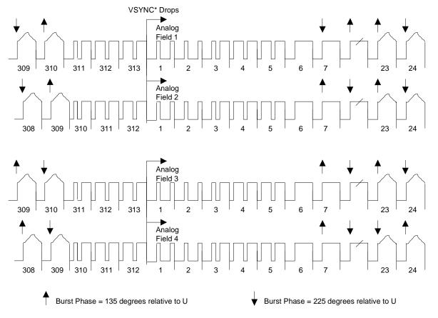
Figure 11. PAL Video Non-Interlaced Progressive Scan Timing
