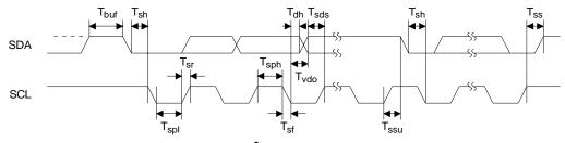
Figure 2. I<sup>2</sup>C Host Port Timing
