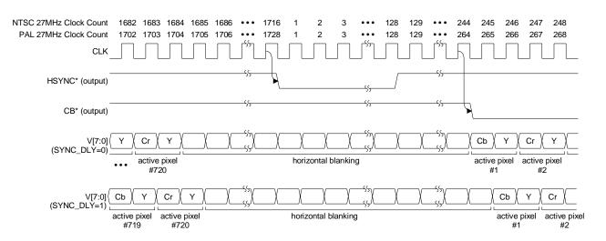
Figure 7. CCIR601 Input Master Mode Horizontal Timing
