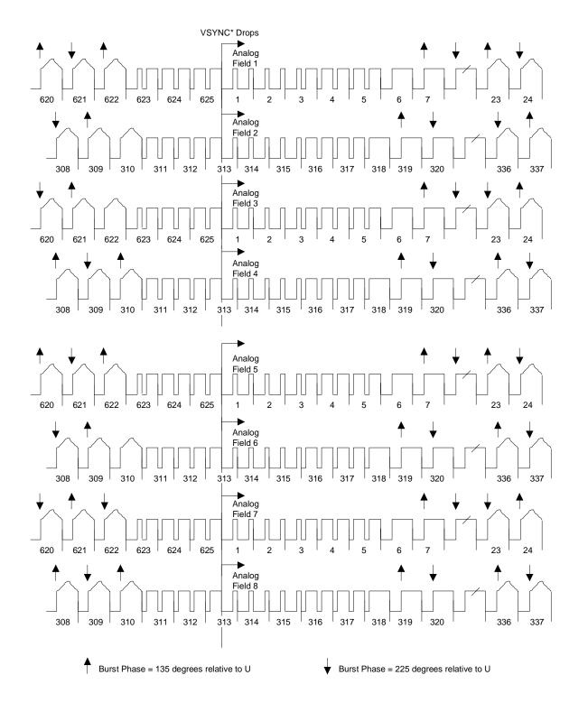
Figure 10. PAL Video Interlaced Timing
