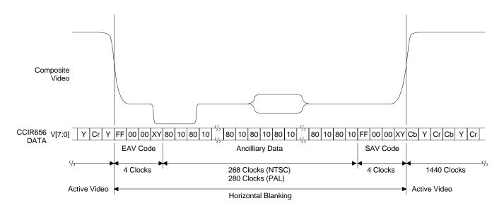
Figure 13. CCIR656 Input Mode Timing
