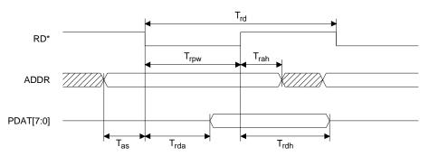
8-bit Parallel Host Port Timing: Read Cycle
