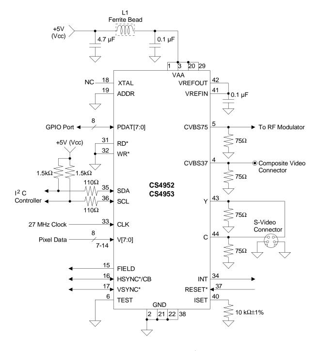
Figure 5. Typical Connection Diagram (I<sup>2</sup>C host interface)
