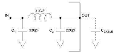
$C_2$  should be chosen so that  $C_1 = C_2 + C_{CABLE}$
