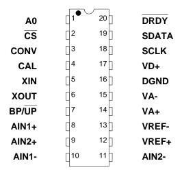
Figure 2. CS5504 Pin Layout
