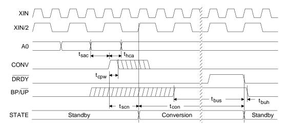
Figure 2. Conversion Timing (Not to Scale)
