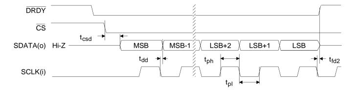
Figure 3. Timing Relationships; Serial Data Read (Not to Scale)
