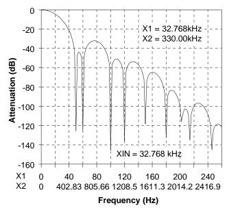
Figure 5. Filter Magnitude Plot to 260 Hz
