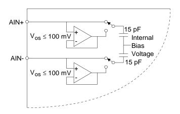
Figure 4. Analog Input Model
