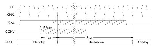
Figure 1. Calibration Timing (Not to Scale)
