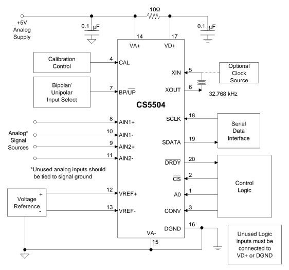
Figure 8. CS5504 System Connection Diagram Using Single Supply
