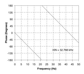
Figure 7. Filter Phase Plot to 50 Hz
