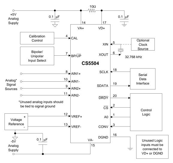
Figure 9. CS5504 System Connection Diagram Using Dual Supplies
