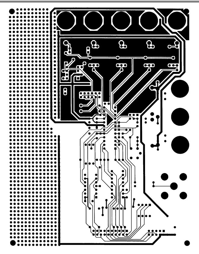
Figure 5. Bottom Trace Layer (NOT TO SCALE)
