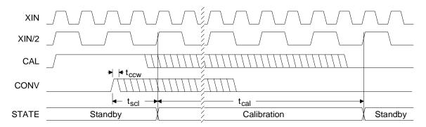
Figure 1. Calibration Timing (Not to Scale)
