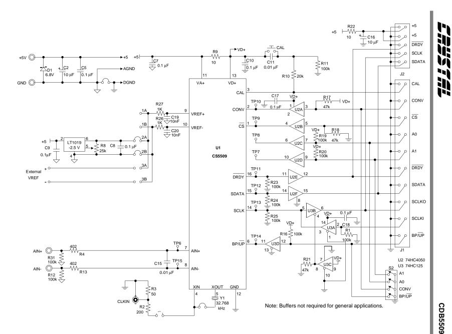
**Figure 1. ADC Connections**
