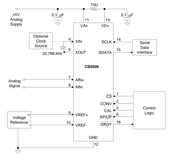
Figure 9a. System Connection Diagram Using a Single Supply
