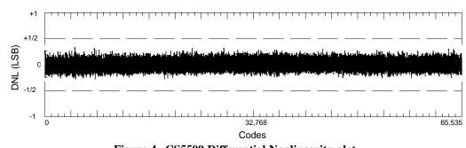
Figure 4. CS5509 Differential Nonlinearity plot.
