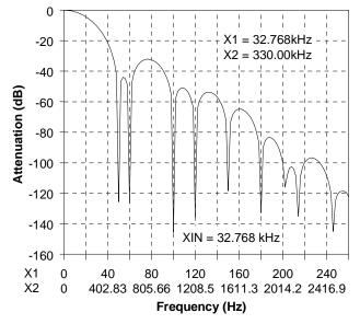
Figure 6. Filter Magnitude Plot to 260 Hz
