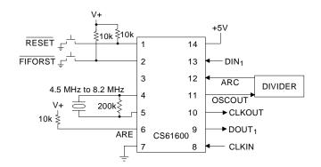
Figure A4. Low Clock Frequency Jitter Attenuation
