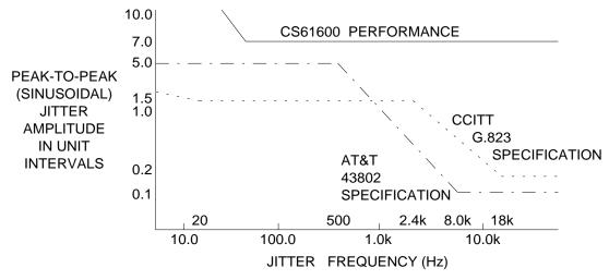
**Figure 4. Input Jitter Tolerance**
