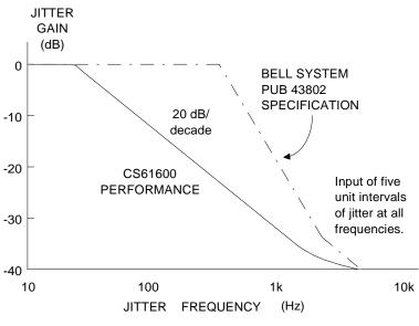
**Figure 5. Jitter Attenuation Characteristic**
