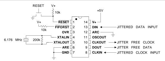
Figure A1. Typical Application Circuit
