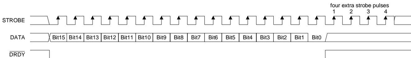
**Figure 4. Microcontroller Interface**
