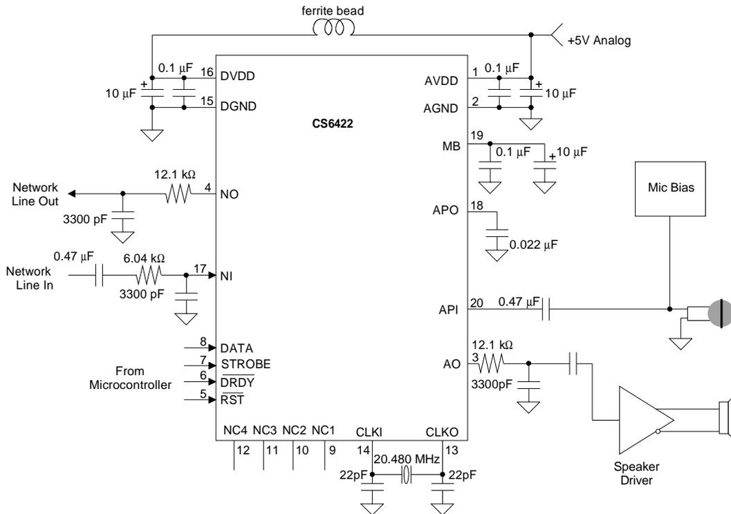
**Figure 1. Typical Connection Diagram (Microphone Preamplifier Enabled)**
