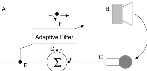
**Figure 7. Simplified Acoustic Echo Canceller Block Diagram**
