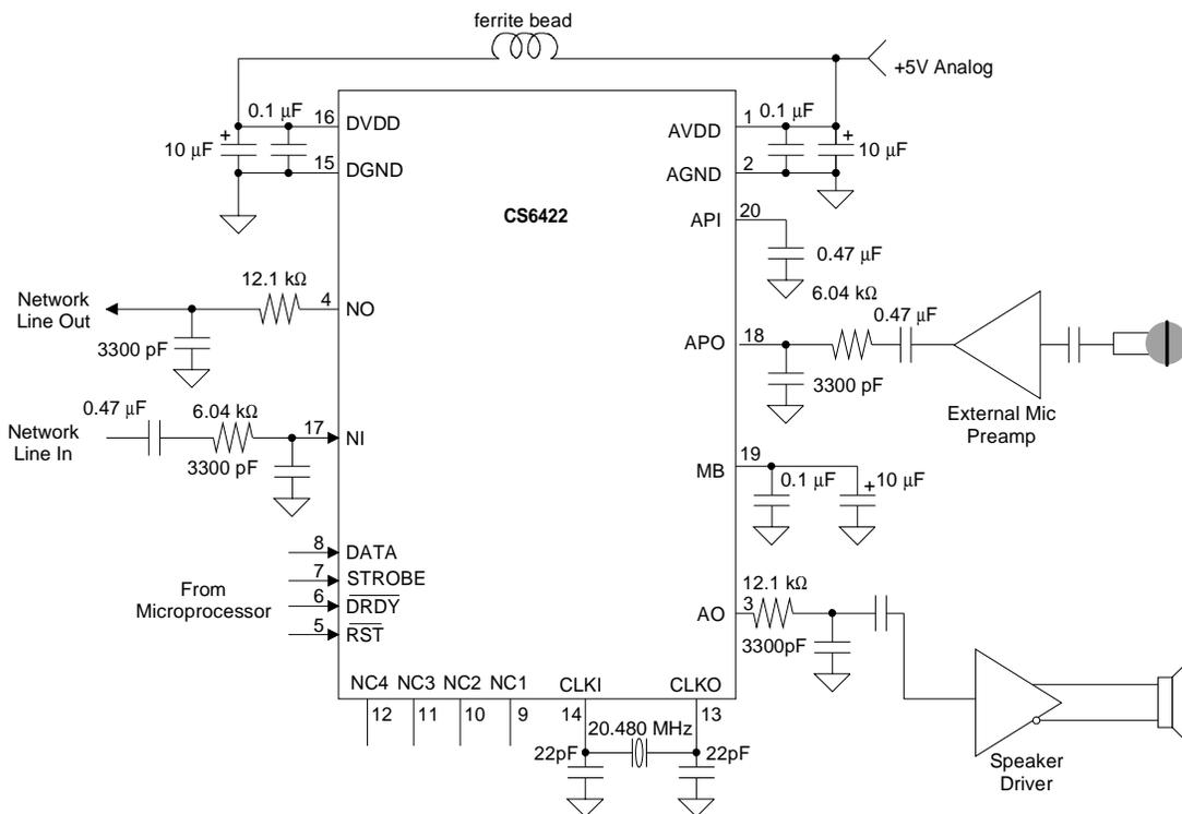
**Figure 2. Typical Connection Diagram (Microphone Preamplifier Disabled)**
