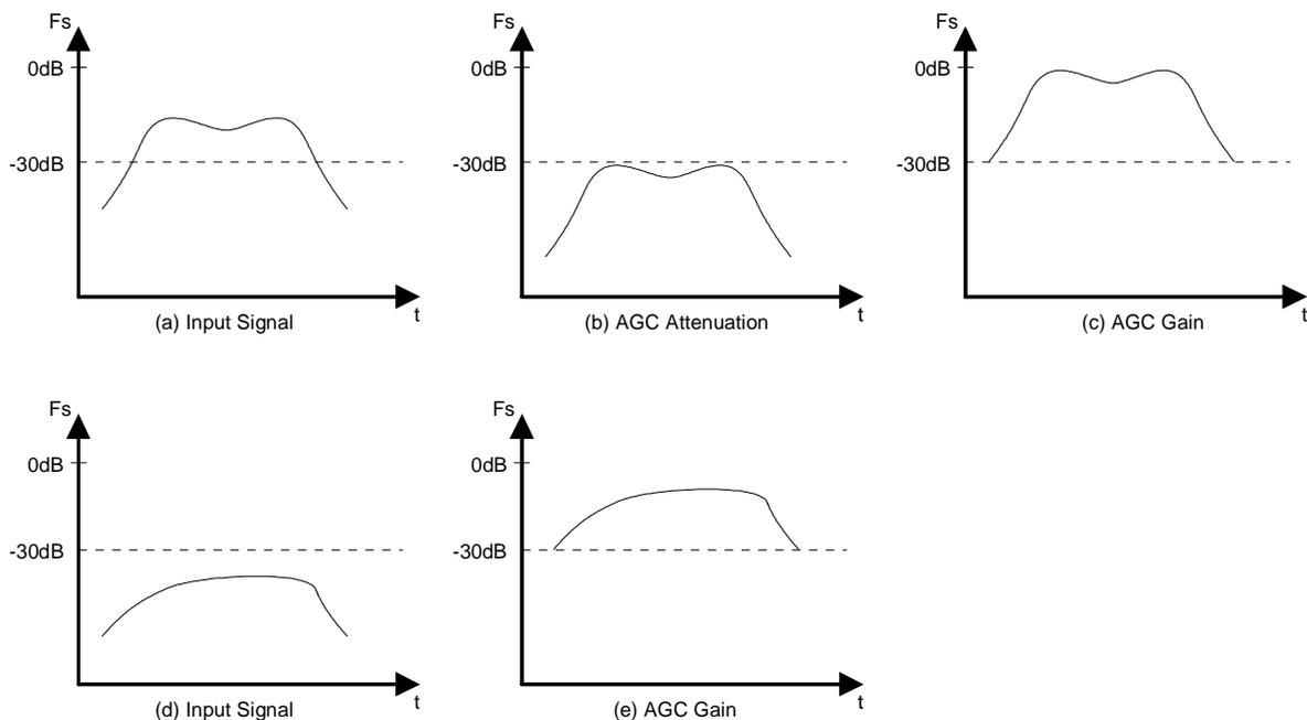
**Figure 8. How the AGC works (TVol = +30 dB)**
