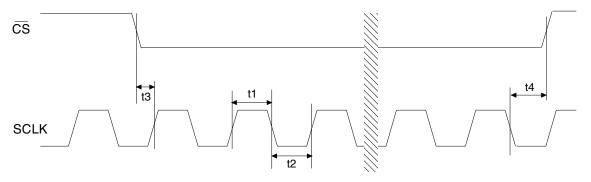
Figure 1. Continuous Running SCLK Timing (Not to Scale)
