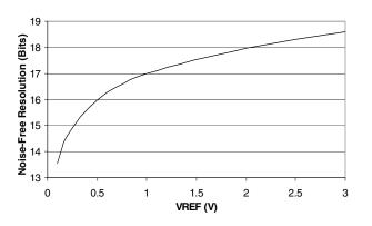
Figure 5. Typical Noise-Free Resolution vs. Voltage Reference Noise-Free Res. = log<sub>2</sub> (Bipolar Span/6.6\*RMS Noise)
