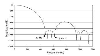
Figure 11. Filter Response (MCLK = 32.768 kHz)
