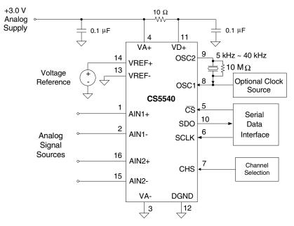
Figure 7. CS5540 Configured with a single +3.0 V Supply
