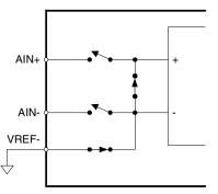
**Figure 9. Self Calibration of Offset**
