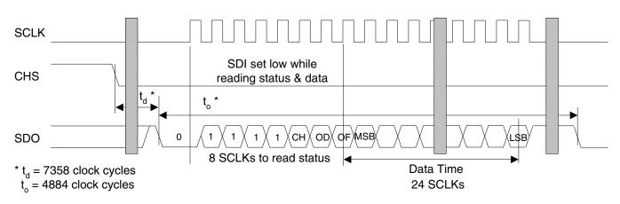
Figure 8. Command and Data Word Timing
