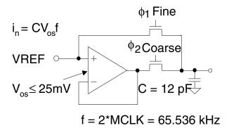
Figure 6. Input model for VREF+ and VREF- pins
