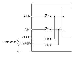
Figure 10. Self Calibration of Gain
