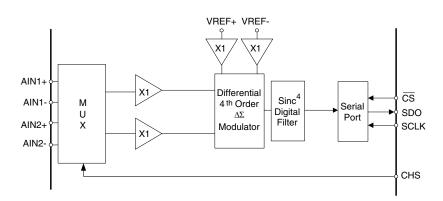
Figure 3. Multiplexer Configuration
