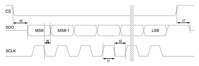
Figure 2. SDO Read Timing (Not to Scale)
