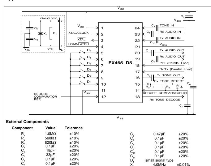
**Note:** The values specified for  $R_1$ ,  $C_2$  and  $C_3$  have been found to be satisfactory when used with a crystal  $(X_1)$  whose equivalent series resistance is  $\leftarrow$  1000 ohms. The crystal manufacturer should be consulted to determine optimum values for different crystals.
