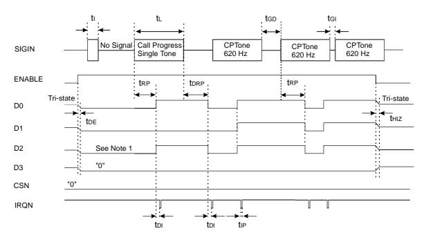
Figure 4 Timing Diagram: Call Progress Tone(s)
