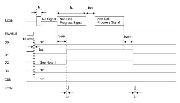
Figure 5 Timing Diagram: Non Call Progress Signal
