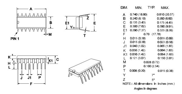
Figure 10 P3 Mechanical Outline: Order as part no. FX663P3
