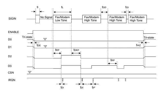
Figure 7 Timing Diagram: Fax/Modem Tones
