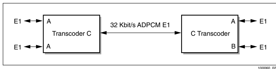
Figure E-2. Single-Board Transcoder Application
