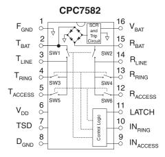
$<sup>^{\</sup>ast}$  Only the CPC7582BA contains the protection SCR.
